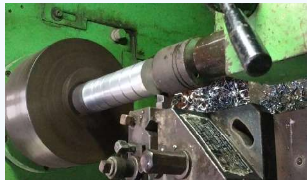
Figure 2 Mild steel workpiece with HSS tool.
