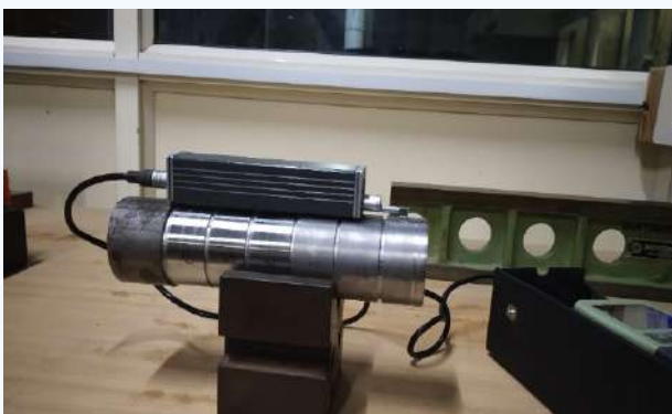
Figure 5 Portable surface roughness tester Surfptest SJ-210 series.
