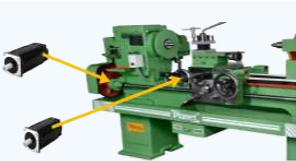
Figure 7 The first motor to the carriage and the second motor to the lead screw of the lathe machine.
