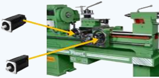
Figure 6 DC motors are directly mounted to the carriage box of the lathe machine.
