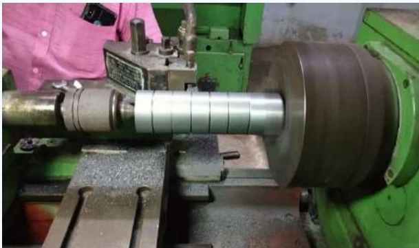
Figure 4 Cast iron workpiece with a carbide tool.
